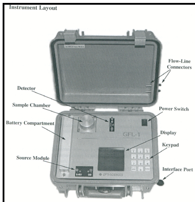
Figure F3.2: GFL-1 Portable Field Fluorometer
