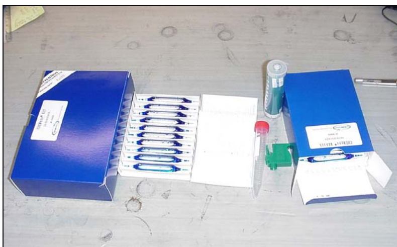
Figure F3.1: CHEMetrics detergent test kit components
