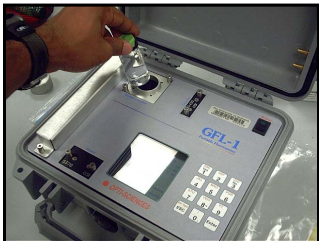
Figure F3.5: Placing Sample into Sample Chamber
